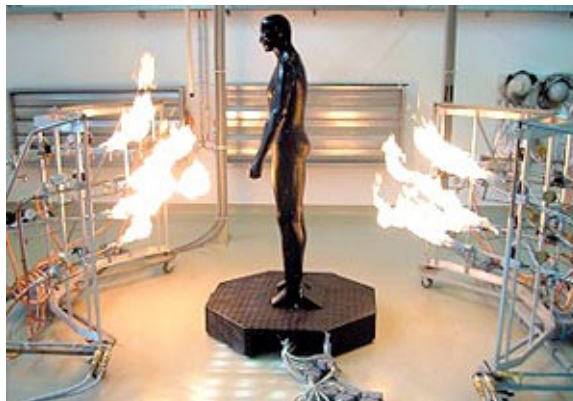
Application to test the heat –resistance of clothing: Thermo-man : Fast thermocouples places on the outside of the special dummy. Digital I/O to check and control the state of the valves of the burners.
